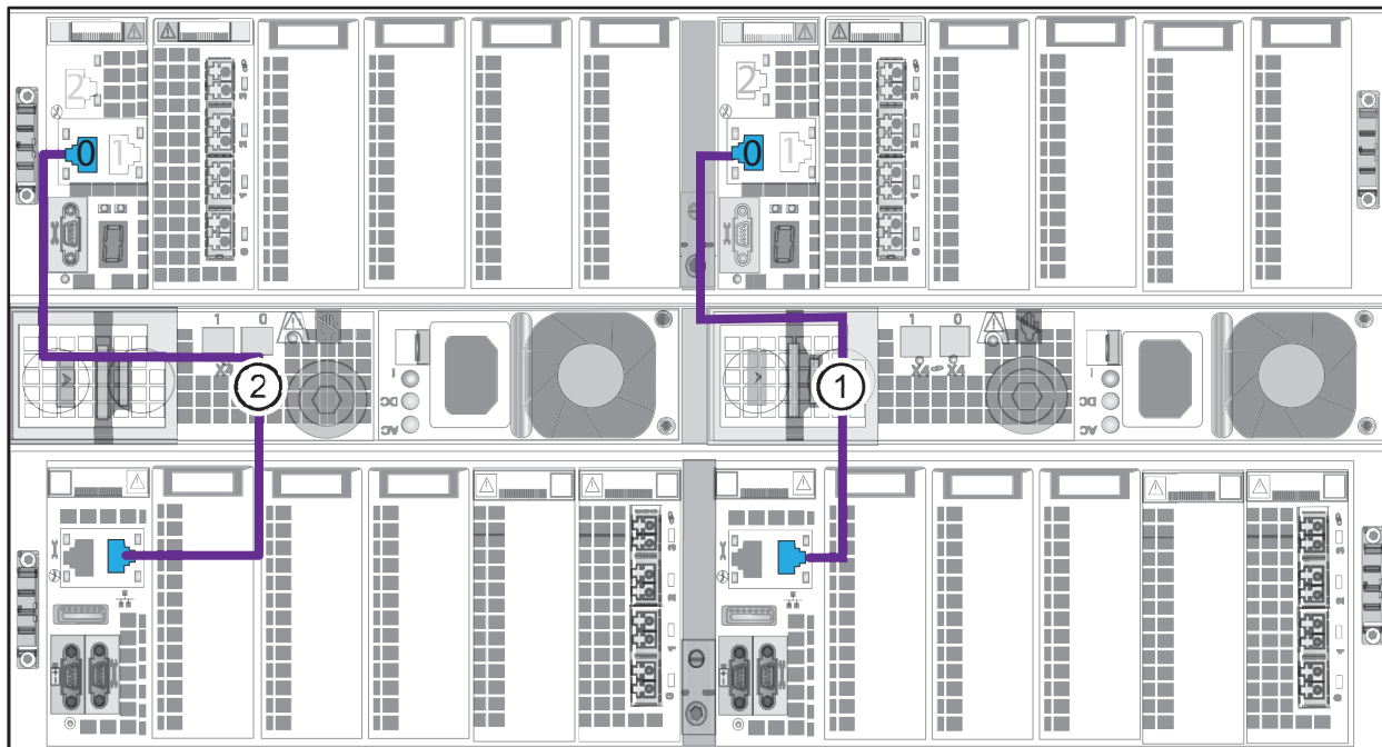
Figure 36 Cabling SPs to blade enclosure 0
