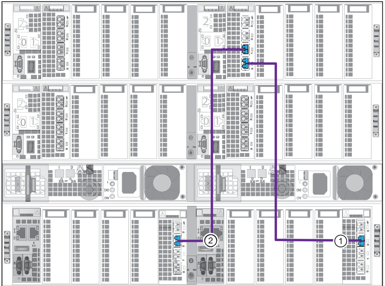
Figure 34 Cable storage processors to blade 4
