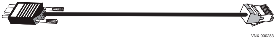
Figure 17 Example of SP A (micro DB-9) SPS (RJ-12) cable
