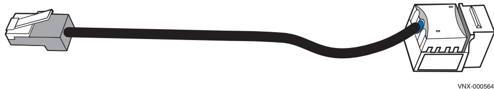
Figure 34 Example of an Ethernet extension (modular plug to modular jack) cable
