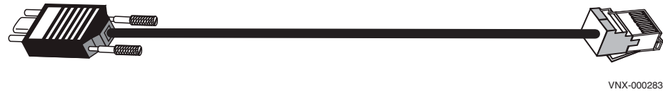
Figure 14 Example of SP A, MGMT A (micro DB-9) to SPS A (RJ-12) cable
