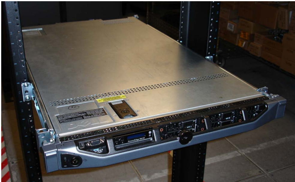
Figure 13. R610 Mounted in the A2 Static Rails (2-post Center Mount Configuration)
