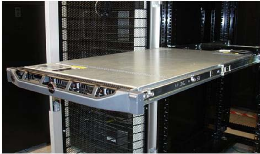
Figure 11. R610 Mounted in the A1 Sliding Rails
