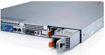
Figure 7. 350W power supply unit
