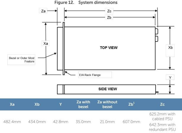
$^{1}$ Zb goes to the nominal back wall external surface where the system board I/O connectors are located.
