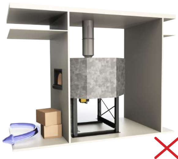
Blocked Air Vent
