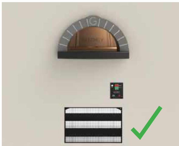
Gozney Classic oven enclosure with adequate venting
