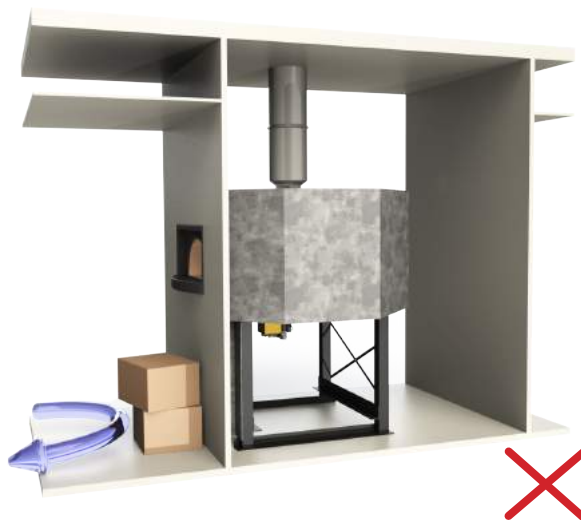
Blocked Air Vent
