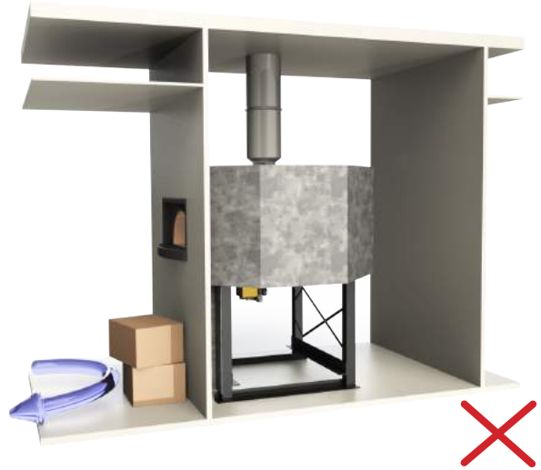
Blocked Air Vent
