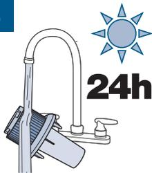
Cyclonic system can be rinsed to clean. Let dry for 24 hours before replacing.
