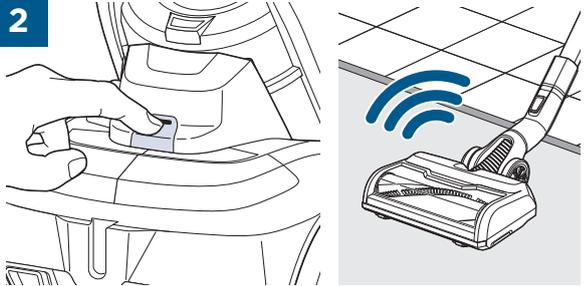
Press Auto Button on back of unit for automatic floor type sensing. The SmartClean canister will detect your floor type and adjust suction as necessary.
