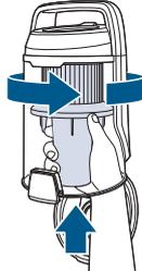
Replace cyclonic system and turn clockwise to lock in place.
