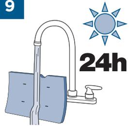
Mesh filter can be rinsed to clean. Let dry for 24 hours before replacing.
