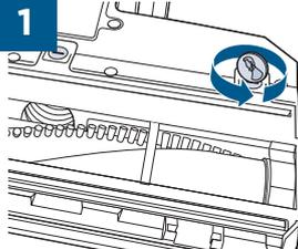
Use a coin to turn screws counter-clockwise to remove the sole plate.
