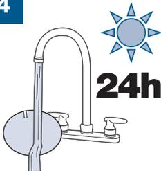
Both filters can be rinsed to clean. Leave to dry for 24 hours before replacing.
