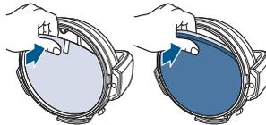
Replace both filters making sure the flat felt filter is inserted first.
