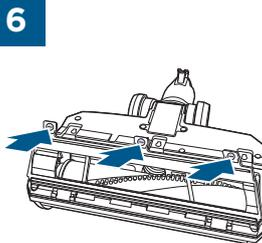
Replace sole plate to the foot. Use coin to turn them to lock into place.
