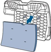
Replace mesh filter in back cover. Make sure all 4 tabs are aligned with their slots in the filter.
