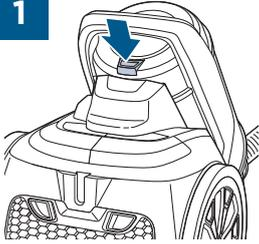
Press Dirt Tank Release Button to remove the tank from the unit.
