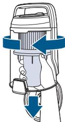
Turn cyclonic system counter-clockwise to release and remove from the tank.
