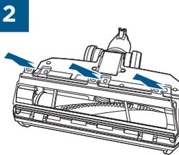
Once screws are unlocked, lift off sole plate.
