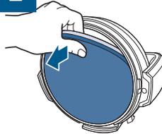
Remove foam filter from the tank lid.
