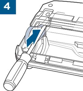
Use a flat head screwdriver to fit the belt over the gear.
