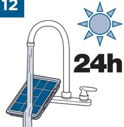
Pleated filter can be rinsed to clean. Let dry for 24 hours before replacing.
