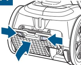
Replace back cover of the unit by pressing the tabs inward to lock in place.
