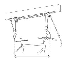
Locate the ceiling joist. Transfer the distance measurement (Step 1) so that the pulleys line up to the correct distance along the joist (Note: It is also possible to mount the pulleys first onto a board which can then be securely mounted to joists as illustrated).
