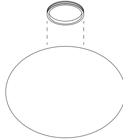
Attach the Shade Washer to the Mushroom Diffuser by aligning the threads and rotating clockwise until firmly in place to seal the connection.
