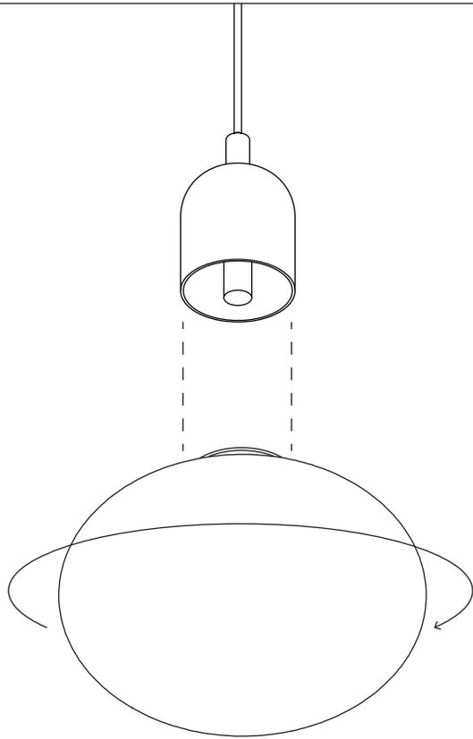
Attach the diffuser to the Shell Pendant Assembly by rotating clockwise until firmly in place to seal connection.
