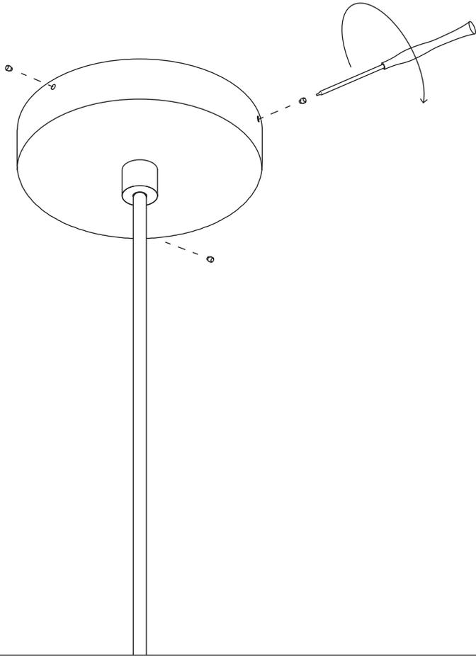
Align the holes of the backplate with the holes of the canopy cover. Secure them in place using the given hex key to twist in the set screws.
