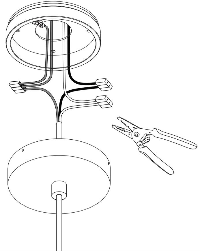
Use the wago clips to connect the fixture's wires to the corresponding wires from the junction box in the wall or ceiling. White is neutral; Black is live; Green/ Yellow is ground. One ground wire will be from the pendant cord, the second wire will be from the canopy backplate, and the third ground wire should come from the junction box. If needed, use a wire stripper to remove 3/8" insulation from each wire before inserting them into the corresponding wago clip.
