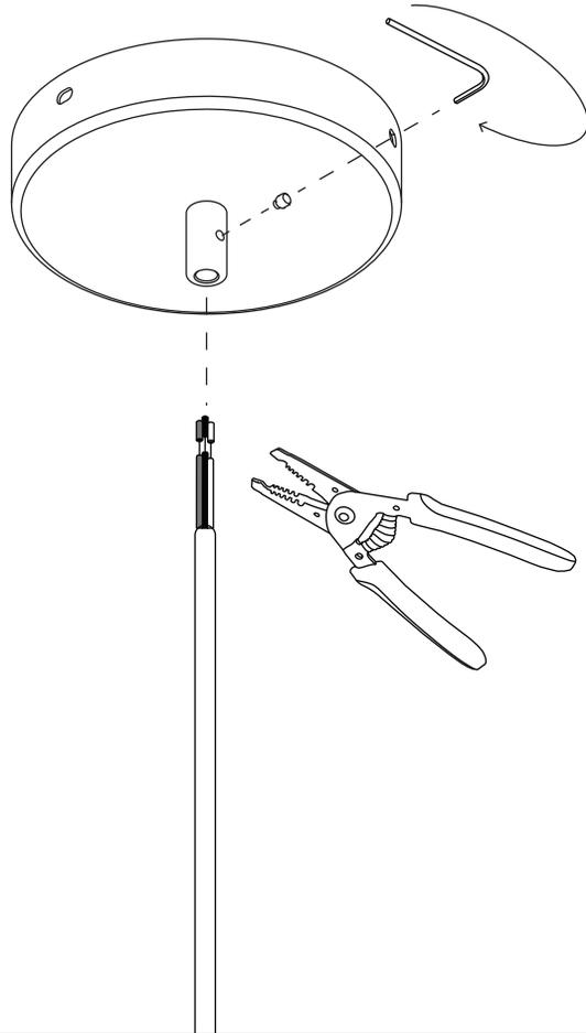
Cut the pendant cord to the desired length using a wire cutter. Then thread the cord through the strain relief attached to the canopy, securing the cord in place by tightening the set screw on the side of the strain relief using the included L-shaped hex key. Please resist the urge to over-tighten; it's not necessary.
