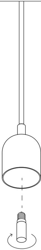
Gently place the Washer over the threaded part of the diffuser.
