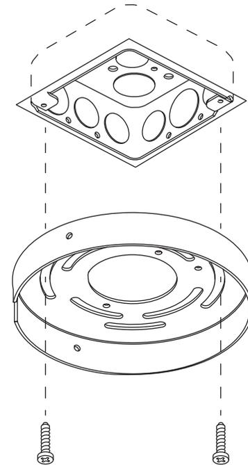
Mount the backplate to the junction box using a phillips head screwdriver to tighten the mounting screws.
