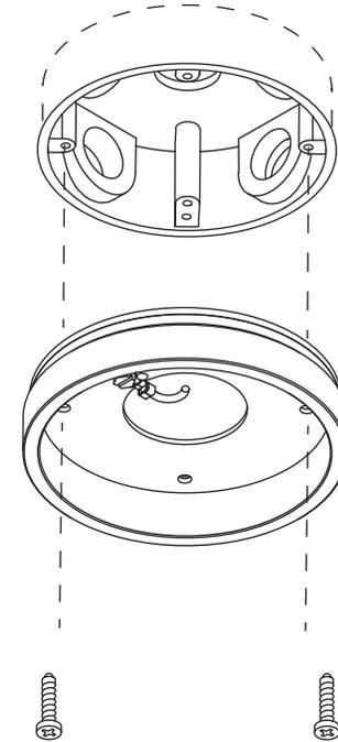
Mount the backplate to the junction box using a phillips head screwdriver to tighten the mounting screws.
