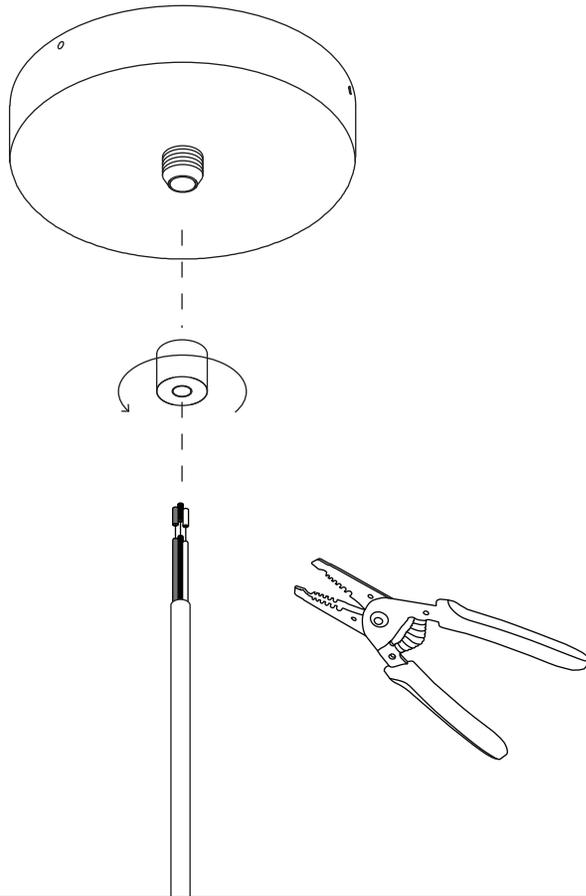
Unscrew the cord cap from the canopy by rotating counter-clockwise. Feed the pendant cord into the cap and through the canopy. Cut the pendant cord to the desired length using a wire cutter. Rotate the cord cap with the cord attached clockwise to secure back onto the canopy.
