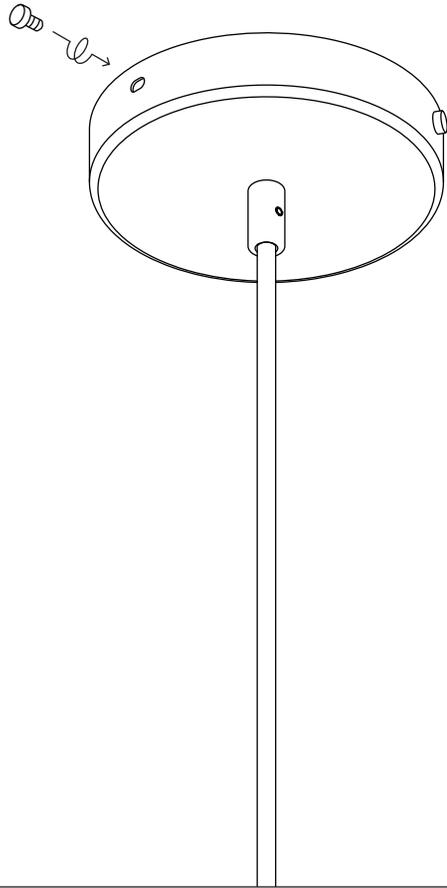
Align the holes of the backplate with the holes of the canopy cover. Secure them in place by twisting the thumbscrews by hand.
