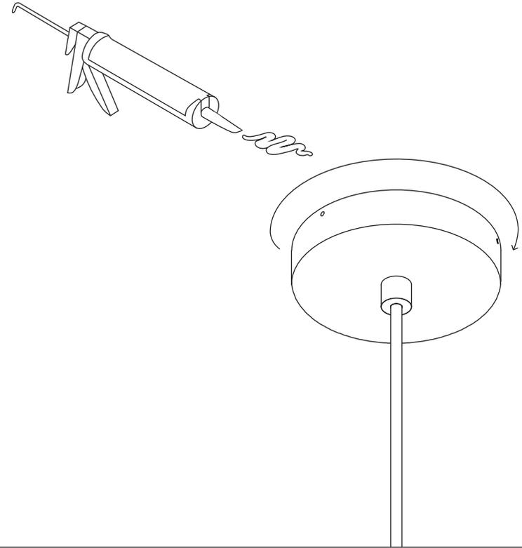
If installing outdoors, carefully apply a bead of silicone caulk between the canopy and the outdoor surface. Smooth the silicone around the light using your finger freshly dipped in a bowl of water.
