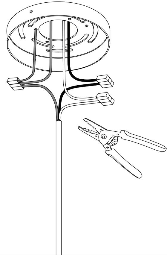
Use the wago clips to connect the fixture's wires to the corresponding wires from the junction box in the wall or ceiling. White is neutral; Black is live; Green/ Yellow is ground. One ground wire will be from the pendant cord, the second wire will be from the canopy backplate, and the third ground wire should come from the junction box. If needed, use a wire stripper to remove 3/8" insulation from each wire before inserting them into the corresponding wago clip.
