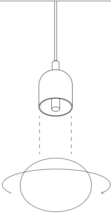
Attach the diffuser to the metal hardware by rotating clockwise until fixed in place. Please refer to the following pages for the Double Puck Pendant, Arundel Orb Pendant, and Arundel Mushroom Pendant.
