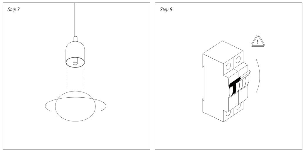
Attach the diffuser to the metal hardware by rotating clockwise until fixed in place. Please refer to the following pages for the Double Puck Pendant, Arundel Orb Pendant, and Arundel Mushroom Pendant. Turn the power back on at the main fuse box or circuit panel you disabled before installation. Turn on the light :)
