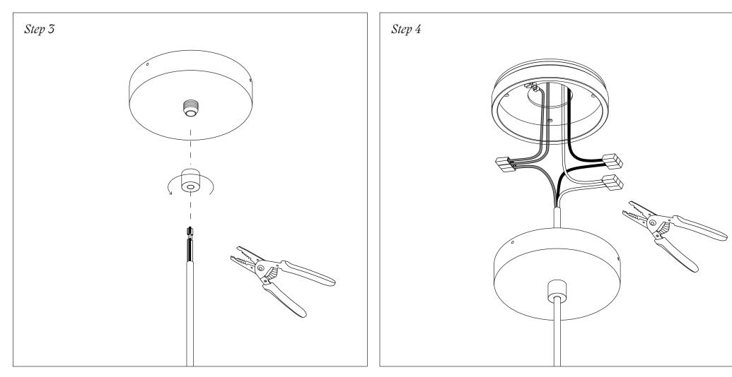
Unscrew the cord cap from the canopy by rotating counter-clockwise. Feed the pendant cord into the cap and through the canopy. Cut the pendant cord to the desired length using a wire cutter. Rotate the cord cap with the cord attached clockwise to secrure back onto the canopy.
