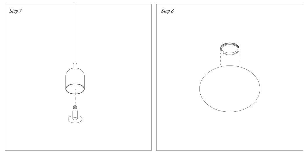
Gently place the Washer over the threaded part of the diffuser.
