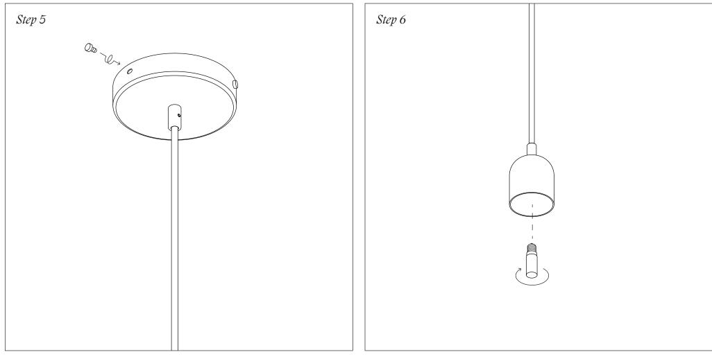
Align the holes of the backplate with the holes of the canopy cover. Secure them in place by twisting the thumbscrews by hand.
