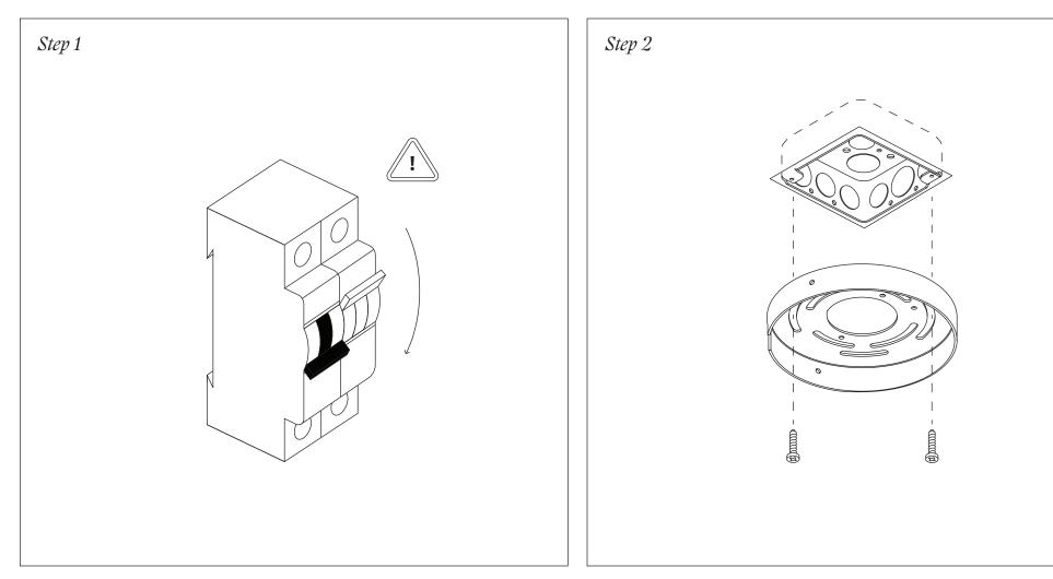
Before beginning installation, turn off electrical power at the main fuse box or circuit panel.
