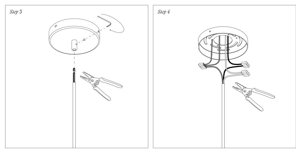
Cut the pendant cord to the desired length using a wire cutter. Then thread the cord through the strain relief attached to the canopy, securing the cord in place by tightening the set screw on the side of the strain relief using the included L-shaped hex key. Please resist the urge to over-tighten; it's not necessary.
