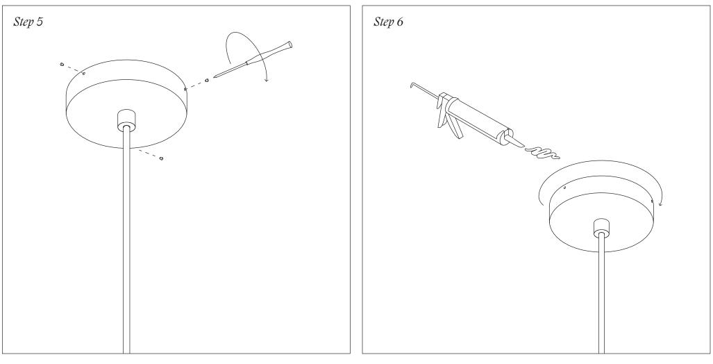
Align the holes of the backplate with the holes of the canopy cover. Secure them in place using the given hex key to twist in the set screws.
