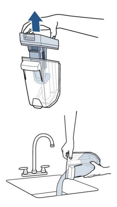
• Remove the filter from the float stack and clear it of debris
