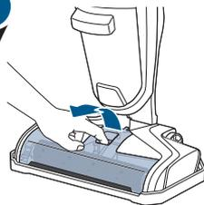
Grasp Brush Window at the front of the window and pull upward to remove.
