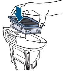
Place Vacuum Filter back into the top of the Dirty Water Tank.
