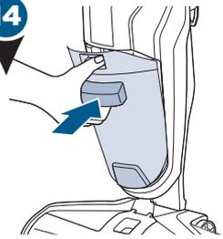
Angle the tank back into body of machine inserting bottom first. Then tilt the top of the tank toward the machine and push into place until you hear a click.
