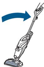
Recline the machine while in storage tray. Allow the machine to run for 10-15 seconds until all water is picked up. Repeat as needed.
