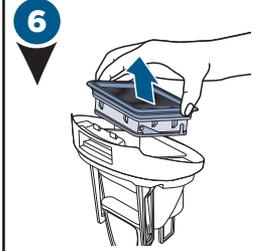
6 Remove the Vacuum Filter and Screen from the top of the Dirty Water Tank by pulling it up.
