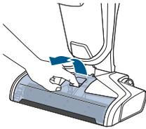
Grasp Brush Window at the front and pull upward to remove.
