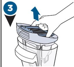
3 Grasp top of Dirty Water Tank in recessed areas on each side of the filter and pull upward to remove the top of the tank.
