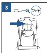
Using a Phillips-head screwdriver, secure the Carry Handle with the screw that's taped to the Upper Handle.
