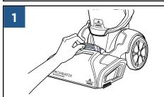
Lift the Accessory Hose Door on top of foot on the front of the machine. The door flips toward the machine to open.
