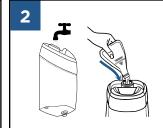
Unscrew the cap from the Clean Water Tank. Add warm tap water to the water fill line. Add desired formula to the formula fill line. After formula is added, secure the tank cap in place.
