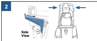
Next, align the Carry Handle with the slots on either side of the base (behind the Power Switch and Cleaning Mode Switch). The Carry Handle will "click" into place.
