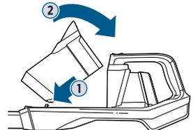
**6.** Put the whole tank into the hand vacuum by guiding the notched out area on the bottom of the tank onto the hook on the hand vacuum. Push into place.
