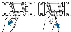
**2.** Insert the tool holders into the side of the Wall Storage & Charging Station. To install the charging cord, remove the power cord clip from the Wall Storage & Charging Station. Insert the charging cord and secure it with the charging cord clip.
