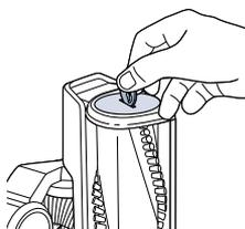
**2.** With a flathead screwdriver or coin, twist the slot on the side of the foot clockwise and pull the Brush Roll out.
