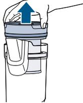
**2.** Grab the top of the tank and pull up. This will activate a wiping feature to remove debris from the mesh filter screen.
