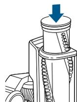
**3.** To replace, push the Brush Roll back in the chamber and twist counter-clockwise with a tool or coin to lock in place.
