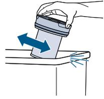
**3.** Fully remove the separator from the tank and tap the mesh screen on the side of the trash bin.
