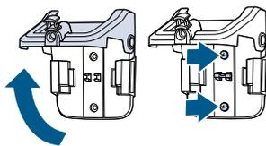
**1.** Open the Wall Storage & Charging Station, use the bubble level to ensure it is level and insert two screws to secure to wall. In order to charge the machine, ensure the Wall Storage & Charging Station is mounted near a wall outlet.
