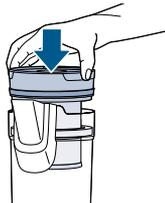
**5.** Slide the separator back into the tank, ensuring the notch is seated into the tank correctly.
