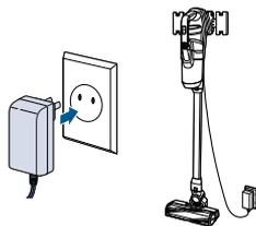
**3.** Plug the power adapter into the wall and place the machine on the Wall Storage & Charging Station for charging. Refer to page 6, "Charging the Battery" for instructions.
