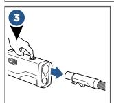
Press release button and disconnect flex hose from the dog bathing tool by pulling straight out. (DO NOT twist tool to remove.)
