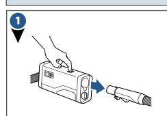
Press release button and disconnect flex hose from the BarkBath™ tool by pulling straight out. (DO NOT twist tool to remove it from the cleaner.)
