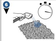
Prime the tool by pointing the nozzle at the microfiber mat and pressing and holding the spray trigger for 15-20 seconds to allow solution to dispense.
