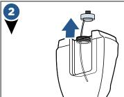
Flip the tank so the black cap is on top and unscrew. Pull up to remove cap assembly from tank.
