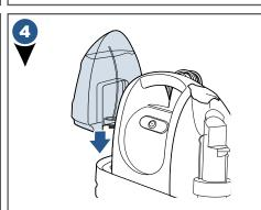
Replace the clean water tank by lining up the grooves on the clean water tank with the vertical guides on the side of the unit. Gently slide it down into position.
