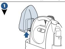
With the machine turned OFF, remove the clean water tank by lifting it straight up and then away from the unit.
