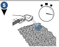
Prime the tool by pointing the nozzle at the microfiber mat and pressing and holding the spray trigger for 15-20 seconds to allow solution to dispense.
