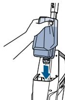
**6.** Align tank with grooves on back of the machine. Slide tank down until you hear a "click".
