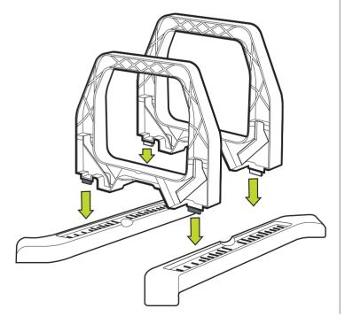
Snap in support arms (Part A) to securely connect base to upright. Ensure uprights are perpendicular to base.
