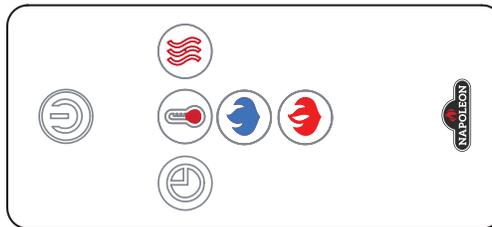
The touch display panel is shown by LED's on the front bottom right of the appliance. The LED's will disappear after 10 seconds of no function change. The main power button will be dim.
