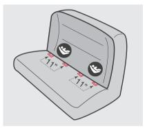
LATCH may be used for spacing larger than 11" ONLY if your vehicle manufacturer allows it.
