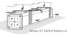
2. Place the outdoor TV face down on a flat surface with a foam board protected. Mount the outdoor soundbar with brackets to the outdoor TV using the 4 provided screws. At least two people are required for installation to avoid any damage due to the heavy weight.
