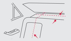
WARNING: CHILD RESTRAINTS MUST NOT BE ATTACHED TO UNSOUND METAL OR TO WOOD, OR SYNTHETIC STRUCTURES. WHEN DRILLING THE 9 MM HOLE DO NOT DRILL THROUGH FUEL LINES, FUEL TANKS, ELECTRICAL WIRING, OR RADIO SPEAKERS. WEBBING STRAPS MUST BE PROTECTED FROM SHARP CORNERS AND EDGES.
