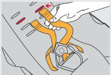
Thread the harness straps through the proper harness slot. Make sure that the straps are not twisted.
