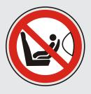
Do not install the child restraint on a vehicle seat that faces either sideways or to the rear of the vehicle.
