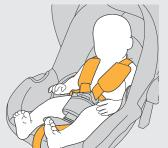
Press the adjuster button on the front centre of the seat, and pull on both shoulder straps to loosen the harness.
