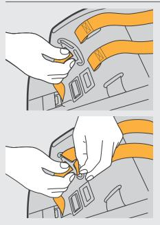
From the rear of the seat, secure the harness strap onto the splitter plate.
