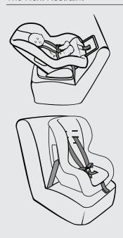
This restraint is suitable for a baby up to approximately 6 months of age. When the baby's shoulders are level with the shoulder height marker (see page 21) they should move to a bigger restraint. The next category of restraint is forward facing and has a six point harness and will be suitable for the child until they are approximately 4 years of age.
