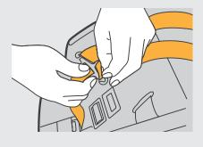
Then take the straps off the splitter plate located at the rear of the seat.
