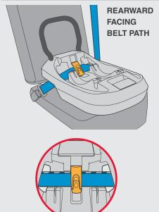
Unlock the vehicle belt lock-off on the base, put the vehicle belt through lock-off and belt slot on the other side, then lock the lock-off.
