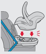
Put the child restraint rear facing on the base, and press it downward. When the child restraint engages securely you will hear a "click".
