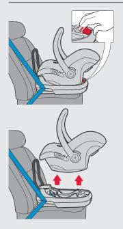
Pull up the easy release lever at the back of the base, and lift the child restraint out.
