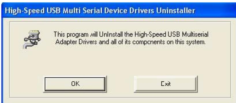
Use the “**Exit**” button to complete the Uninstaller utility. No need to restart the PC, unless prompted by the OS. The driver can also be uninstalled from **Control panel – Add / Remove Programs**. Select the “High-Speed Multi Serial Compound Device” from the Add / Remove panel
