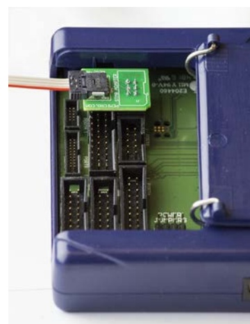
Figure 3-21: STM8 Adapter: 1) Bottom, 2) Top, 3) Connected To 6-Pin Header of Cyclone_Universal (Adapter Sold Separately)
