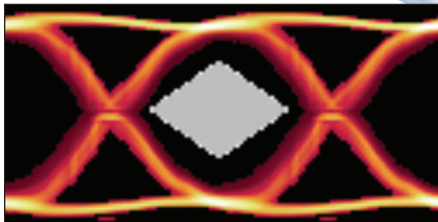
Passing eye-diagram 10 Gbps USB Type-C to USB Type-C cable.
