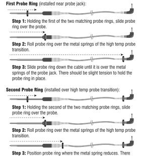
should be slight tension to hold the probe ring in place.
