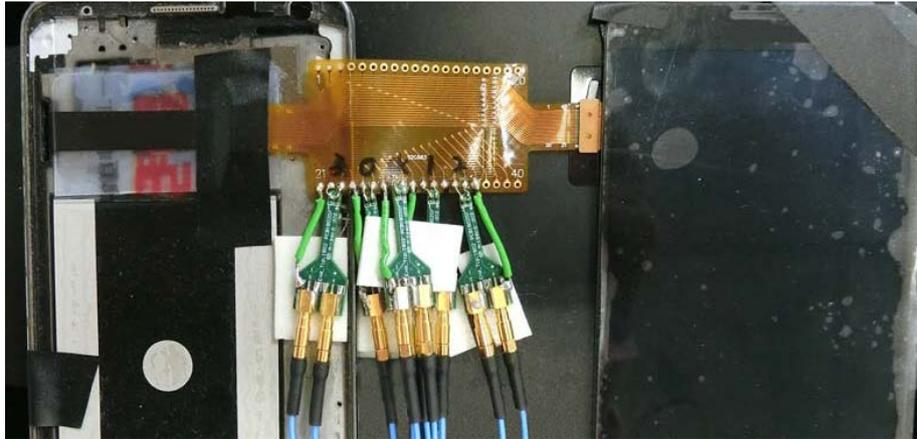
※ End-tip R1/R2 resistor is 1kΩ/0402 which can be replaced if it breaks.
