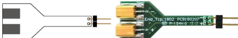
Note: Use hot melt adhesive to reinforce the End-tip.
