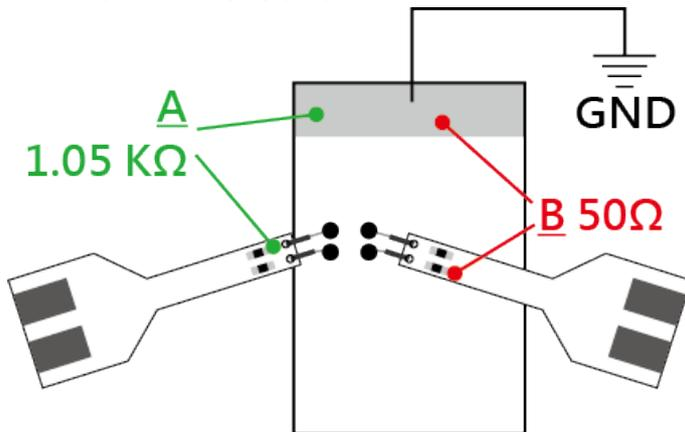
Check point **A**: End-tip resistor front to ground, **green line** ==> no sound from a multimeter.
