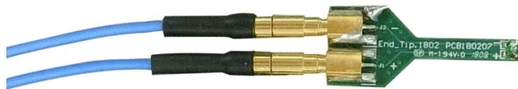
**Step 2: Weld the End-tip to the DUT after Step 1.**
