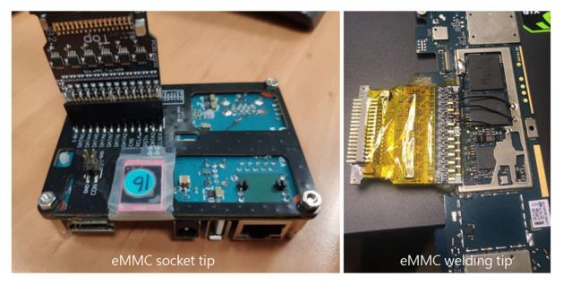
\* Suggestion : The bonding wire distance is about 3cm (the shorter the better), and 100~75 ohm resistance can be added for anti-reflection to improve the measurement quality.
