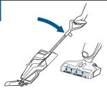
Recline the body of the machine backward to start the Brush Roll spinning. To stop the Brush Roll spinning, you will need to stand the machine upright.
