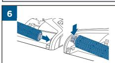
Replace Brush Roll by inserting the Brush Roll end into the right side of the foot. Then lock the pull tab into place by pressing downward.
