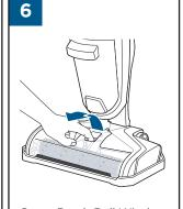
Grasp Brush Roll Window at the front of the window face and pull upward to remove.
