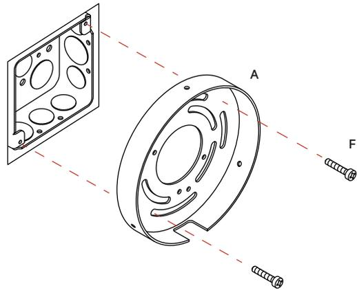
**Step 3:** Use the wago clips (F) to connect the fixture's wires to the corresponding wires from the junction box in the wall or ceiling. White is neutral; Black is live; Green/ Yellow is ground. One ground wire will be attached to the backplate (A), the other ground wire should come from the junction box. If needed use a wire stripper to remove 3/8" of the insulation from each wire before inserting them into the corresponding wago clip.
