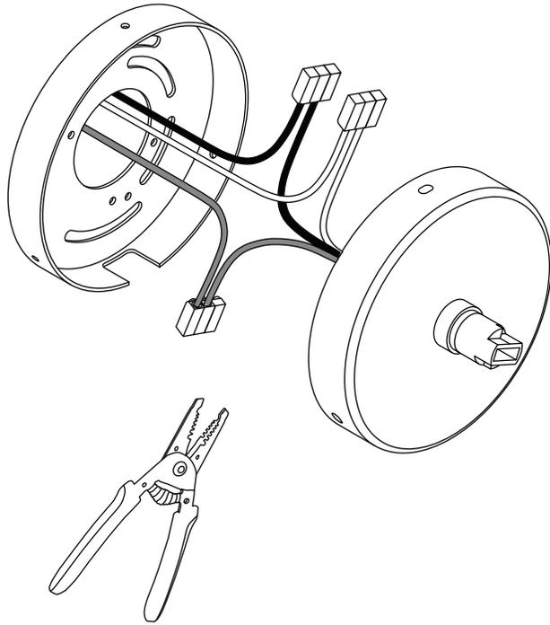
Use the wago clips to connect the fixture's wires to the corresponding wires from the junction box in the wall or ceiling. White is neutral; Black is live; Green/ Yellow is ground. One ground wire will be from the fixture backplate, and the other ground wire should come from the junction box. If needed, use a wire stripper to remove 3/8" insulation from each wire before inserting them into the corresponding wago clip.
