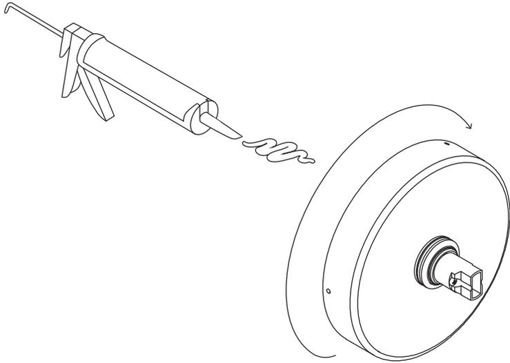
If mounting outdoors, carefully apply a bead of silicone caulk between the G9 Surface Mount and the outdoor surface. Smooth the silicone around the light using your finger freshly dipped in a bowl of water.
