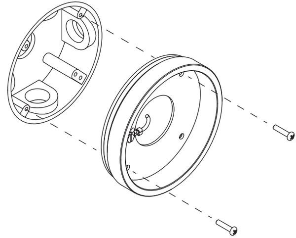
Mount the backplate to the junction box using a phillips head screwdriver to tighten the mounting screws.
