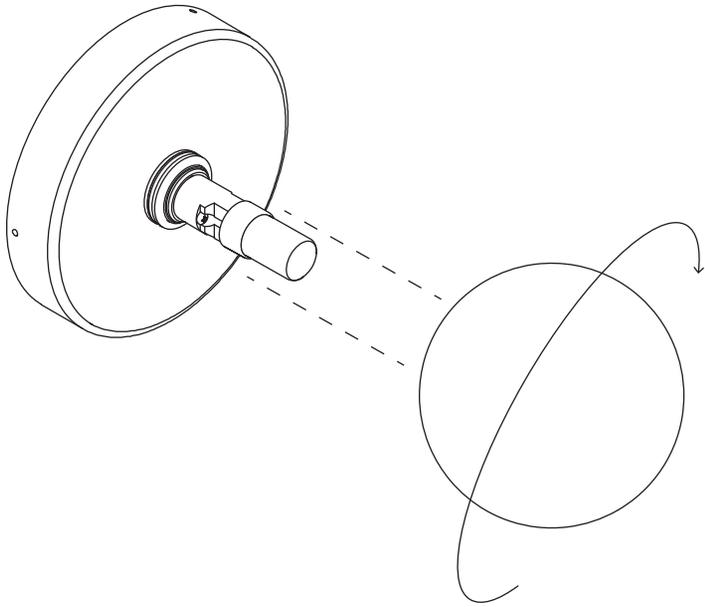
Attach the diffuser to the metal hardware by rotating clockwise until firmly in place to seal connection.
