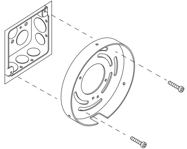
Mount the backplate to the junction box using a phillips head screwdriver to tighten the mounting screws.
