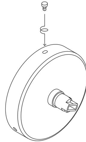
Align the holes of the backplate with the holes of the canopy cover. Secure them in place by twisting the thumbscrews by hand.
