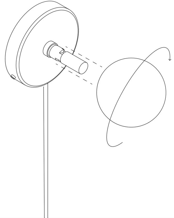
Attach the diffuser to the metal hardware by rotating clockwise until fixed in place.
