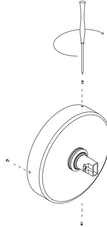
Align the holes of the backplate with the holes of the canopy cover. Secure them in place using the given hex key to twist in the set screws.
