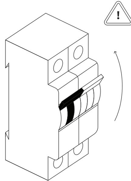
Turn the power back on at the main fuse box or circuit panel you disabled before installation. Turn on the light :)
