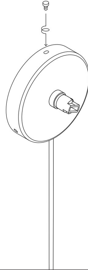
Align the holes of the backplate with the holes of the canopy cover. Secure them in place by twisting the thumbscrews by hand.
