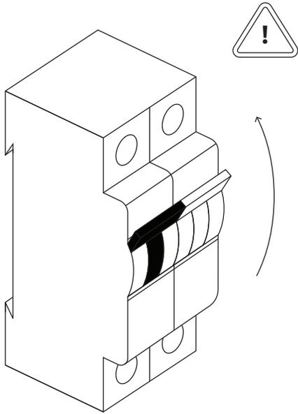
Turn the power back on at the main fuse box or circuit panel you disabled before installation. Turn on the light :)
