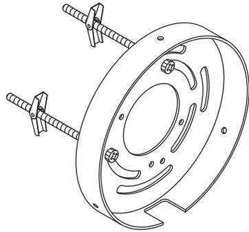
Mount the canopy backplate to the wall using anchors appropriate for your wall material (not provided). Consult a qualified professional if needed.
