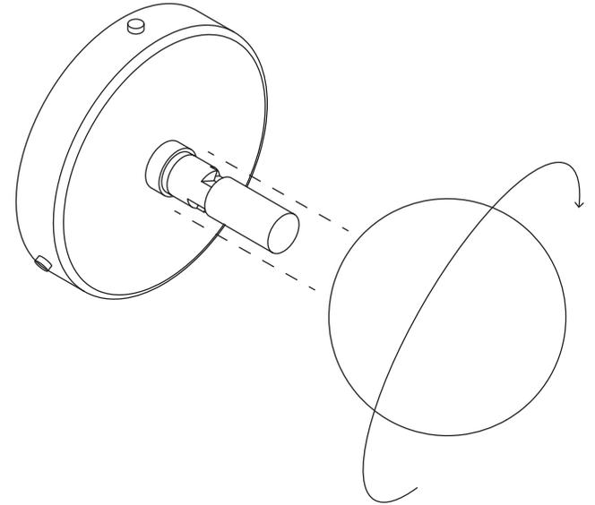
Attach the diffuser to the metal hardware by rotating clockwise until fixed in place.
