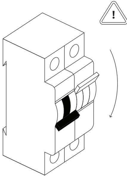
Before beginning installation, turn off electrical power at the main fuse box or circuit panel.
