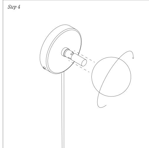
Push the lightbulb into the socket.
