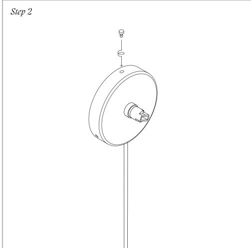
Mount the canopy backplate to the wall using anchors appropriate for your wall material (not provided). Consult a qualified professional if needed.
