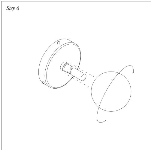
Push the lightbulb into the socket.
