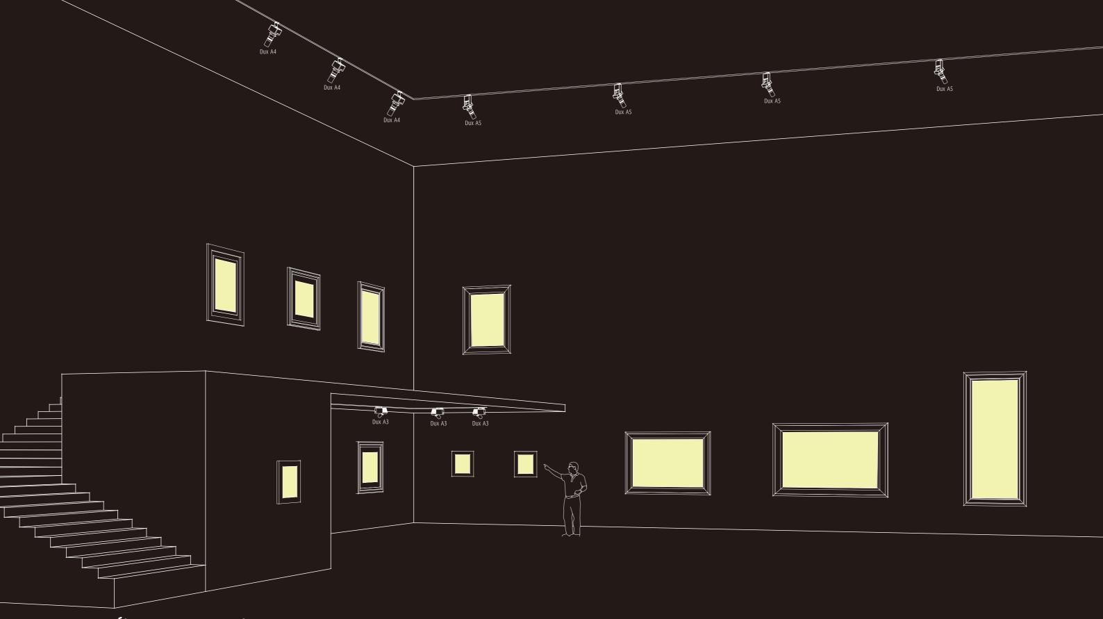
Dux A4 fine art projector Focus on painting, feature the art, capture details. Let every idea shine brilliantly. Distance from 3m to 5m, beam angle from 12°, 18°, 28° to 39° of accurate lighting.
