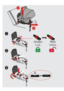
Remove the child seat from the isofix base: first move the child seat carry handle to the upright position (1). Locate the red pull handle on the front edge of the isofix base and pull outwards (2). Lift the child seat up and away from the base.
