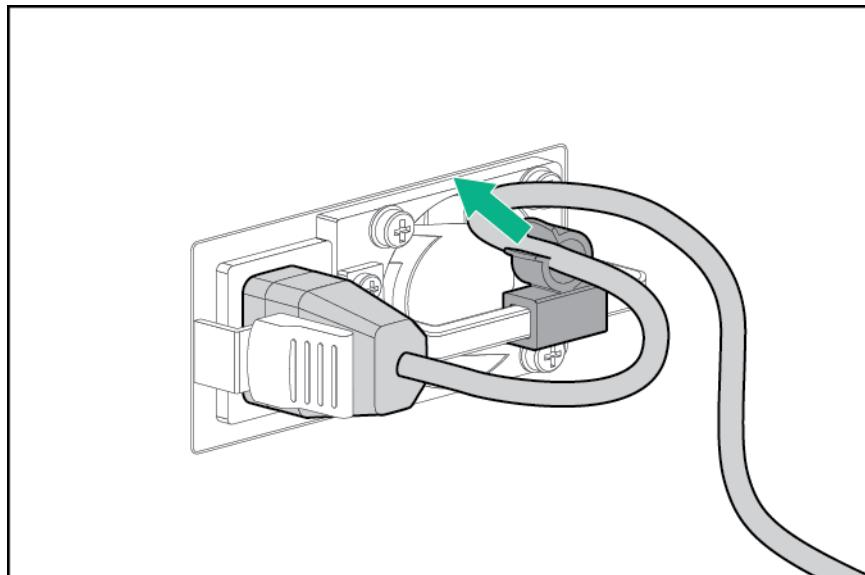
3. Remove the strain relief clip from RPS and retain the clip for future use.
