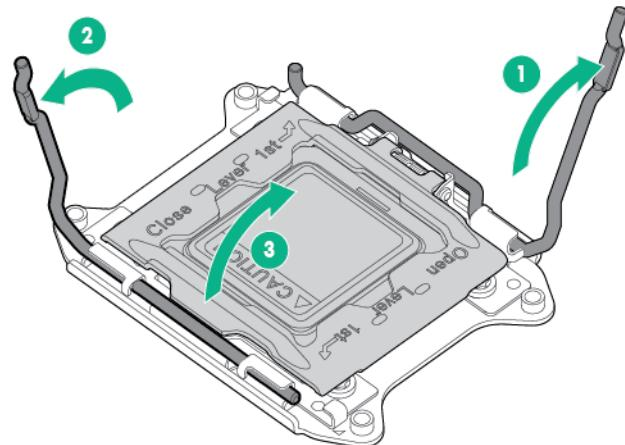
3. Remove the clear processor socket cover. Retain the processor socket cover for future use.
