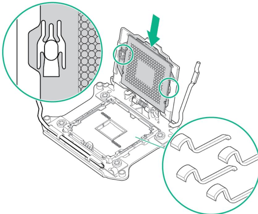
5. Close the processor retaining bracket. When the processor is installed properly inside the processor retaining bracket, the processor retaining bracket clears the flange on the front of the socket.
