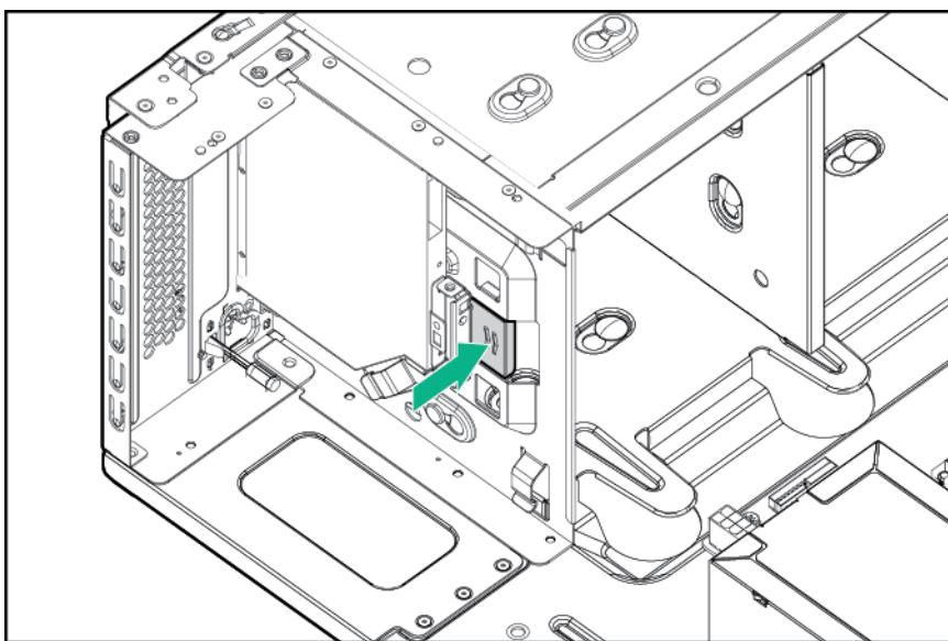
11. Remove the optical drive and disconnect the cable from the rear of the drive.
