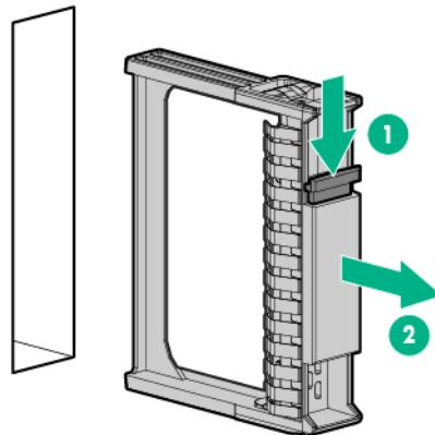
To replace the SFF drive blank, while pressing the release latch, slide the component into the bay until it is fully seated.
