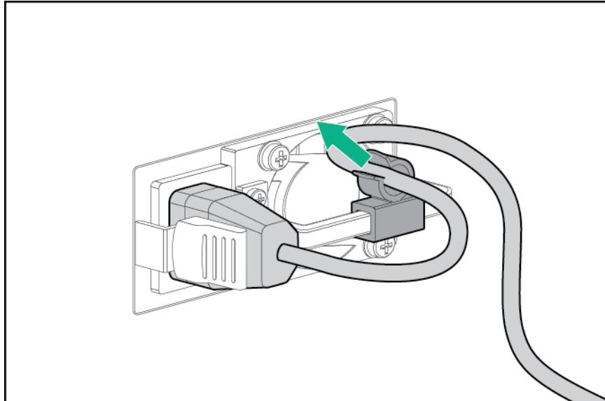
3. Remove the strain relief clip from RPS and retain the clip for future clip.
