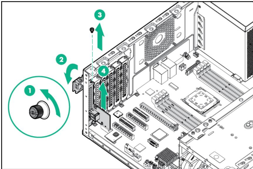
To replace the component, reverse the removal procedure. After installing the new dedicated iLO management module, enable the dedicated iLO connector ("Enabling the dedicated iLO management module" on page 60).
