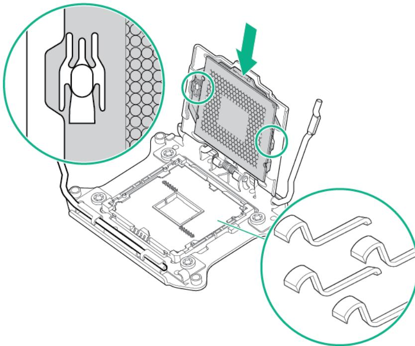
△ **CAUTION: THE PINS ON THE SYSTEM BOARD ARE VERY FRAGILE AND EASILY DAMAGED.** To avoid damage to the system board, do not touch the processor or the processor socket contacts.
