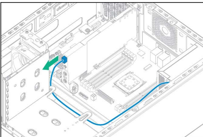
8. Remove the GPU with the supporting holder from slot 1:
