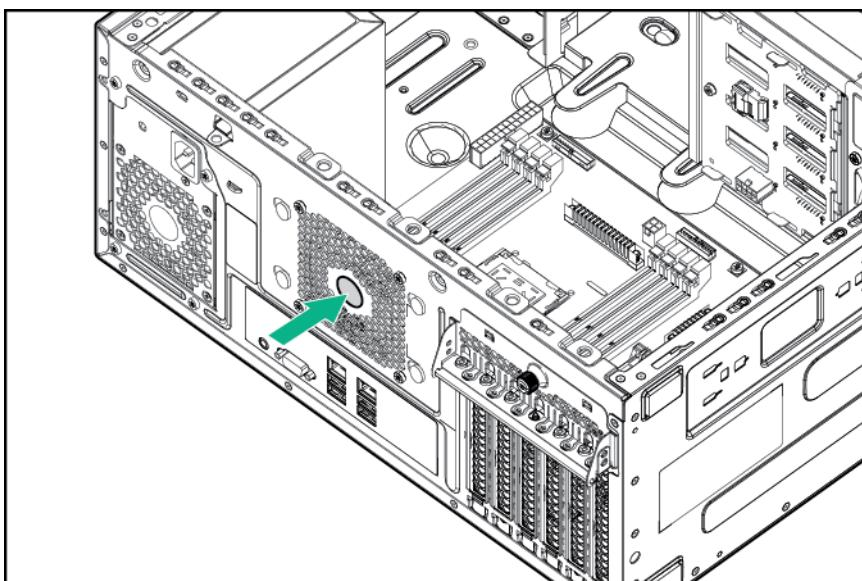
8. Remove the 92 × 38 mm system fan module.
