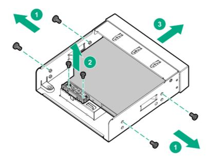
To replace the component, reverse the removal procedure.
