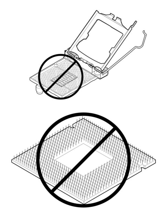
12. Hold the processor by the edges, and then lift it out of the socket.
