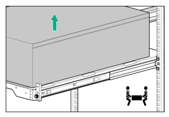
7. Place the server on a flat, level surface with the access panel facing up.
