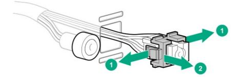
11. Remove the front I/O assembly from the rear panel.
