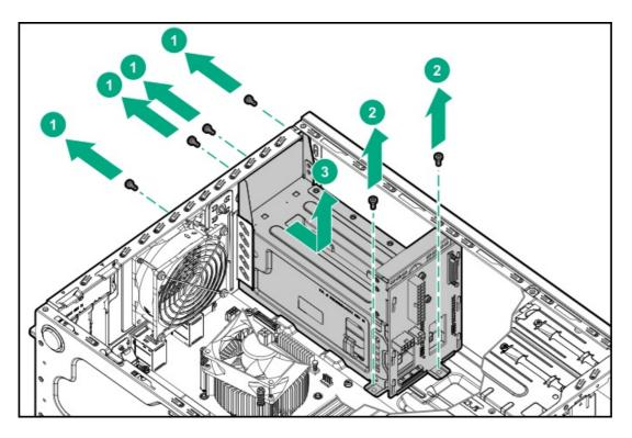
11. Remove the Flexible Slot power supply backplane.
