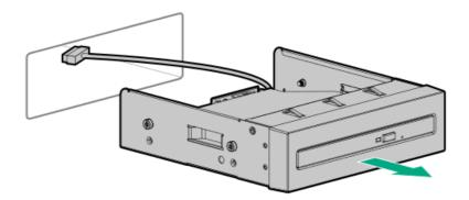
10. Remove the optical drive from the optical drive cage.
