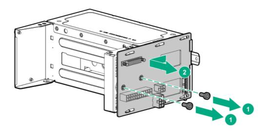
To replace the component, reverse the removal procedure.
