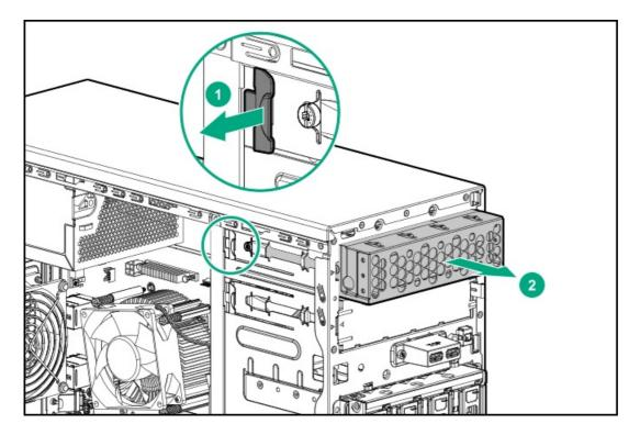
**11.** Remove the screws and slide out the drive from the drive enablement assembly.
