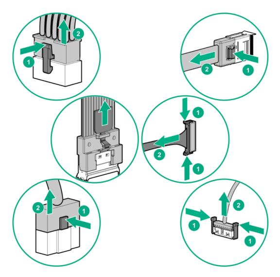
• Remove cables that are no longer being used. Retaining them inside the server can restrict airflow. If you intend to use the removed cables later, label and store them for future use.
