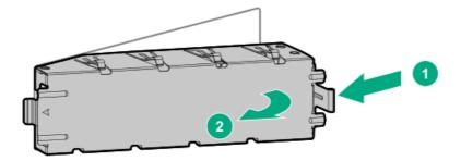
To replace the component, insert the tab on the blank into the slot on the media bay.
