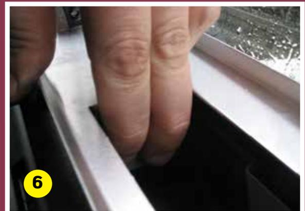
Offer up the base plate to the dash, sliding the tabs inside the ashtray aperture. The taller upright fold should align with the windscreen side of the dash. Press the tabs firmly into place by bending them back under the dash trim as far as possible.
