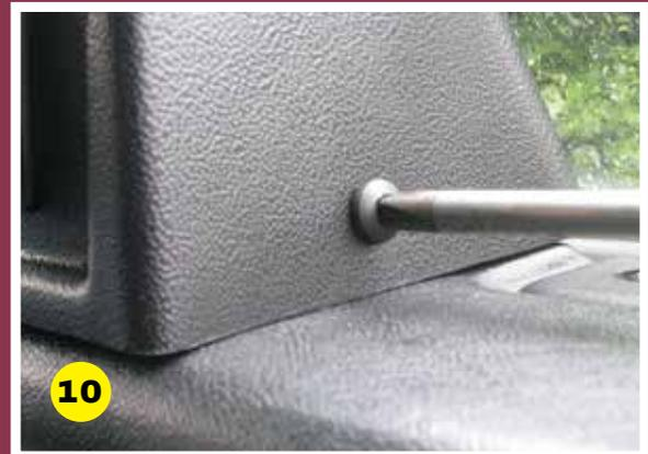
Remove the Pod and drill the holes with a 4.5mm drill. Take the spire clips and slide over the tabs on the end plate. The smooth face of the spire clips should face outwards. Position the pod over the mounting frame and secure using the short screws provided. **JOB DONE!**
