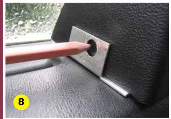
Position the Pod over the base plate keeping one side of the fixing plates outside of the Pod. Mark a fixing hole slightly towards the top of the hole (to account for the thickness of the base plate). Repeat the procedure for the opposite side of the console.
