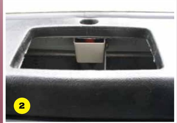
Remove the ashtray from the top of the dashboard. The ashtray is secured with a spring clip at each side. Route your wiring through this aperture.
