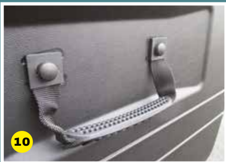
Position handle to suit your preference. Tighten fixing screws. Fit screw caps.
