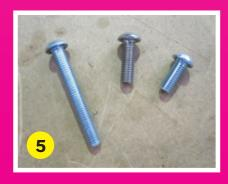
Fit the rear medium sized (25mm) fixing bolts inside the wide end of the rails as illustrated right. This is the rearmost fixing.
