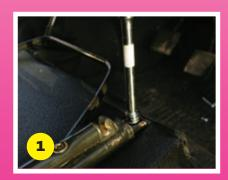
Slide the seat fully forwards to access the rearmost mounting bolts.
