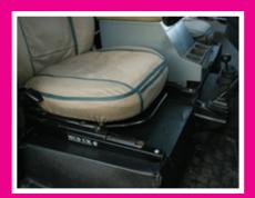
Note that on the Factory fitted *Premium Seat* option (identifiable by their integral headrest) the rearmost seat fixing closest the cubby box uses a stud fixing fitted with a nut rather than a bolt.
