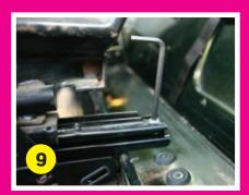
Fully tighten all of the remaining fixings including the front MUD Rail fixing into the seatbox.
