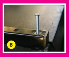
Replace your seat frame on top of the MUD Rails and fix in place using the four remaining short (16mm) bolts.
