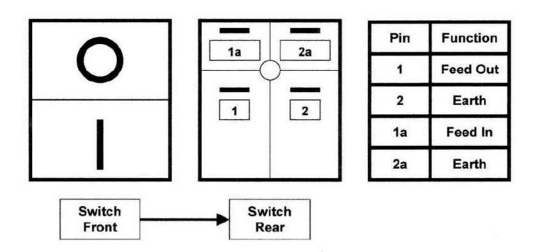
Only one earth connection is required on the switch. Use either terminal 2 or 2a for the earth.
