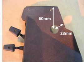
On the heater control end panel the mini vents are not a tight fit when placed in the 22mm holes. A 22mm hole is needed in order for the flanged end of the mini-vent to pass through the panel. We recommend packing out the tube by wrapping the tube where it slots through the hole with insulating tape (below).
