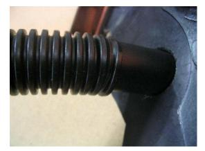
Attach the trunking onto the DefenderVENT off the vehicle before fixing the DefenderVENT into the dashboard. The trunking is a push fit into the large rubber grommet within the dash tray.
