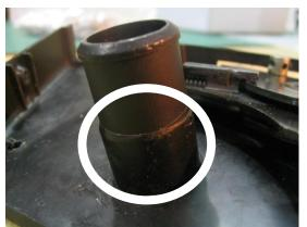
Push the trunking onto the mini-vents. Be patient- they are a tight fit! There is no need to push the trunking to the base of the mini-vent. Secure the Mini-Vent with the pipe clip supplied as below (left).
