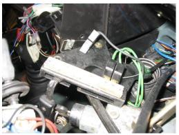
Remove the heater speed control from the end of the dash binnacle. When removing the end panel containing the temperature and vent direction heater controls, remove the three screws on the side and top of the panel first. Ease the panel away from the end of the dash and remove the two screws located immediately above and below the slide controls. Take care to retrieve the two plastic spacers on the heater control assembly highlighted above.
