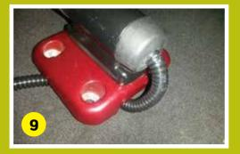
Create a hole in the bottom of the dust cap to route wiring to the back of the hinge.
