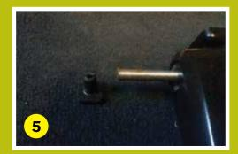
Drill the end of the mirror ball with an 8mm drill.
