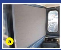
The self-adhesive pad that fits within the front side panel will need reducing in length by approximately 10mm. Cut to size before removing the backing
