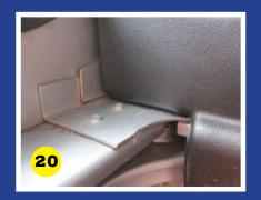
The panel needs to sit down snug on top of the internal roof gutter lip.
