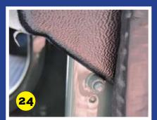
Locate the recessed indicator marks for the fixing positions and drill fixing holes using a 6mm drill bit.
