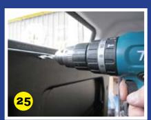
Use the small fir tree fasteners for the upper gutter rail fixings.
