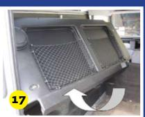
The panels are a tight squeeze over the spot welds in the rear corner.
