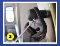
Remove seat-belt bolt with 11/16 or 17mm spanner or socket.
