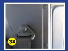
Replace the seatbelt fixing and trim cap.
