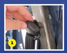
Remove the plastic cap from the seat-belt bracket to expose the seat-belt fastener.
