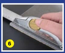
On a vehicle with a standard full height loadspace bulkhead-trim back the plastic as illustrated on the right. Follow the cut lines moulded into the plastic.
