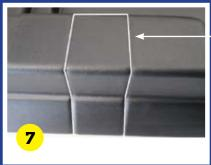
lines. If your vehicle is fitted with a MUD bulkhead removal bar trim back the section illustrated
