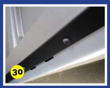
Drill the front fasteners in place into the B pillar on the hardtop using a 6mm drill bit.
