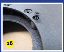
Ensure the side panel trim slides behind the headlining. Watch out for any wiring behind the headlining.
