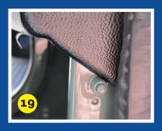
Locate the recessed indicator marks for the fixing positions and drill fixing holes using a 5.5mm drill bit.
