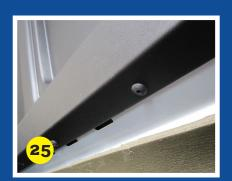
Drill the front fasteners in place into the B pillar on the hardtop using a 5.5mm drill bit.
