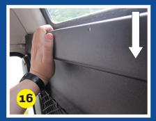
Peel back the door seal rubber and ensure the trim panel fits around the front corner of the door opening.
