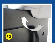
The panels are a tight squeeze over the spot welds in the rear corner.
