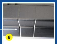
Try to achieve as snug fit as possible around the bulkhead. A file is useful for tidying up the cut edges of the plastic.
