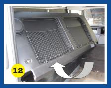
Ensure the side panel trim slides behind the headlining. Watch out for any wiring behind the headlining.
