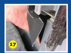
Trim the plastic with a sharp knife if necessary to achieve a snug, flush fit.
