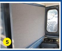
Thoroughly clean the hardtop side panels so that the self adhesive foam pads will stick. Peel away the backing.
