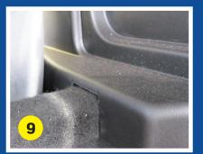
Use a 2.5mm drill to drill the fixing holes for the storage net countersunk screw fasteners.
