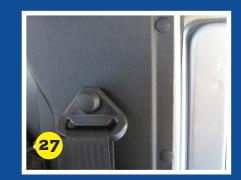
Replace the seatbelt fixing and trim cap.
