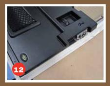
Mark the position of the door handle onto the plastic trim and drill a 10mm hole for the grab handle fixing bolt. Ensure the bolt hole aligns with the rivnut in the door frame.
