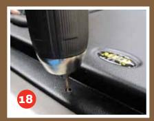
Refit the grab handle using the new socket headed bolt provided. Use a 4mm hex Allen Key.
