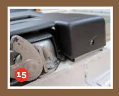
The fir tree fasteners are a push fit.
