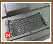
When you've marked the screw holes take care not to snag the netting in your drill when drilling the fixing holes.
