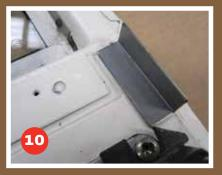
Note how the upper fixing plates fix to the door tapering inwards to follow the rear door outline.
