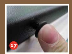
Fix the lower portion of the trim panel to the door frame using the same fitting technique with the rivets. Remember to attach to a solid rust free section of the door frame.
