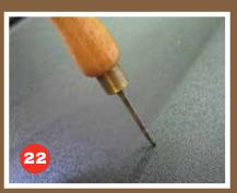
Drill through the trim using a 3mm drill bit.
