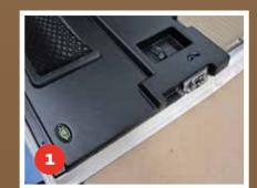
Check the moulding for clearance around the rear door hinge fasteners. Because the positioning of the hinge is adjustable you may need to trim the plastic trim to clear the nuts.
