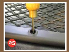
Plug the fixing holes with the plugs provided.
