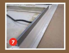
Position and drill the fixing holes in a rust-free area of the door frame! Use a 3mm drill for the fixing screws. Enlarge the holes in the brackets with a 4.5/5mm drill to allow the fixing screw to pass through the bracket.
