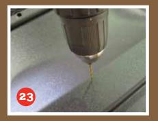
Reposition the net over the fixing hole and screw the net into the door panel with the supplied screws. Align the other screw holes, mark and drill.
