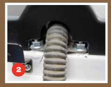
Check clearance around the door check strap. When fitting to a series vehicle you may need to trim a larger section of the plastic away in order to clear the Series style rear door check strap.
