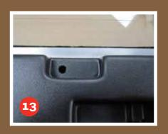
Once you are satisfied the door trim fits snugly around the mounting frame you can now begin to secure the panel. Using a 6mm drill bit drill through the plastic trim into the angled brackets.
