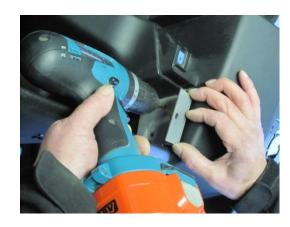
3. Secure mounting bracket using the 2 x self-tapping screws.
