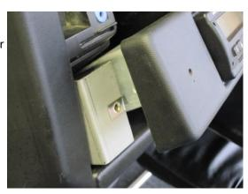
9. Use the plastic washers with the fascia fixing screws.
