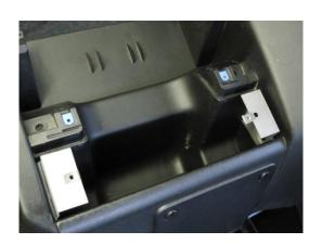
5. Slide the 2 x spire-clips onto the mounting brackets.
