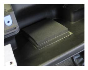
8. Connect wiring to your DIN unit and place the fascia plate over the mounting brackets.
