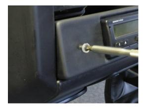
10. Tighten the 2 x fascia fixing screws.
