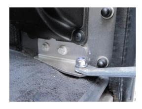
6. Tighten the two fixing bolts.
