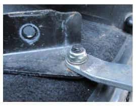
4. Replace the original fixing bolts. Do not tighten fully yet.
