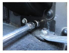
3. Use the new 13mm nut and bolt supplied for the check-strap. Tighten just enough allowing the door to open and close freely.
