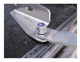
5. Before tightening the fixing bolts, check clearance on B-pillar to prevent damage to the door.
