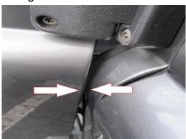
2. Remove the nut on top of the hinge check strap.
