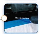
Be sure to keep the drill straight as to not bore out the holes.
